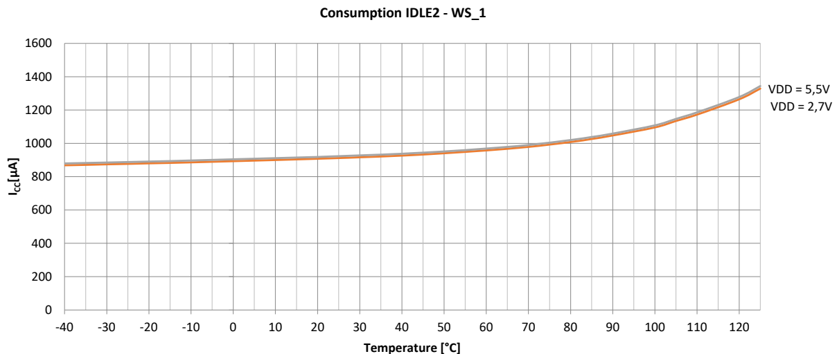
Figure 43-2. Power Consumption at Over Temperature in IDLE Mode (typical Values for guidance only, not characterized over process / voltage)
