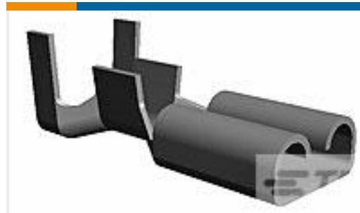
TE Part #170037-2 187 FASTON, REC., 20-16 AWG, TPBR
