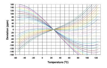
AT Cut Crystal Frequency versus Temperature Typical Performance:
