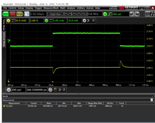
Figure 11. Load Transient, \pm 5\text{ mA} , V_{IN} = 5\text{ V} , C_{IN} = 1\ \mu\text{F} , C_{OUT} = 1\ \mu\text{F} , 50\text{ mV}/\text{div}
