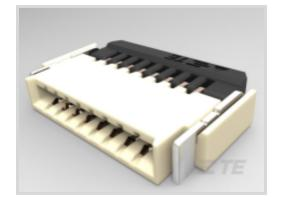
Centerline (Pitch): .5 mm Mating Retention Type: Zero Insertion Force (ZIF) PCB Mount Orientation: Right Angle Contact Mating Location: Dual Side Termination Method to PCB: Surface Mount
