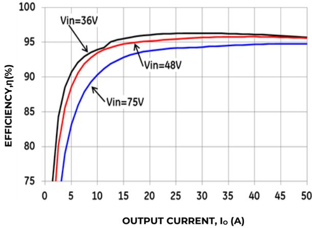
Figure 1. Typical Converter Efficiency vs. Output Current.
