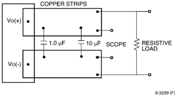
Note: Use a 1.0 μF ceramic capacitor and a 10 μF aluminum or tantalum capacitor. Scope measurement should be made using a BNC socket. Position the load between 51 mm and 76 mm (2 in. and 3 in.) from the module.
