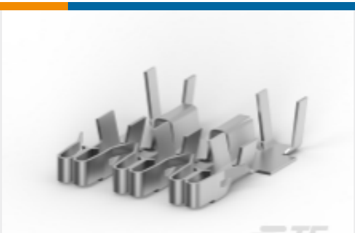
TE Part #881572-2 BUSBAR,STAMPED,CUSN4,0.4MM,3 POSN
