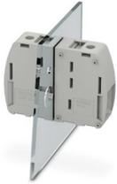
Panel feed-through terminal block, connection method: Screw connection with tension sleeve, Screw connection with tension sleeve, number of positions: 1, load current: 232 A, connection direction of the conductor to plug-in direction: 0 °, width: 25 mm, color: gray. Outer terminal half with screw flange
