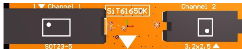
Figure 4. Time Machine socket card SiT6165DK. Supports SOT23-5 package (5-pin) and 3.2 mm x 2.5 mm (4-pin and 6-pin) packages.
