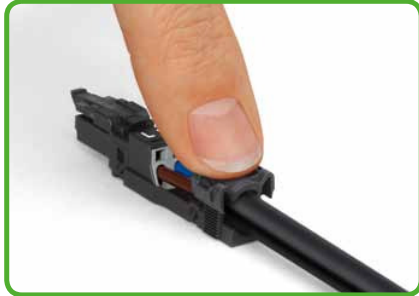
Push down strain relief clamp by hand.
