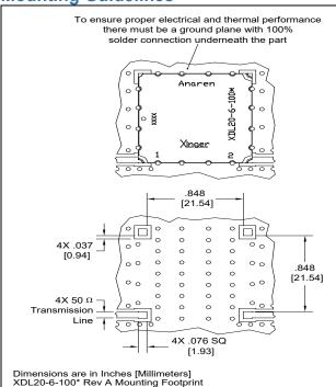
In order for Xinger surface mount delay lines to work optimally, there must be  $50\Omega$  transmission lines leading to and from all of the RF ports. Also, there must be a very good ground plane under the part with a number of plated thru holes to ensure proper electrical performance. If any of these conditions are not satisfied, insertion loss, average delay and VSWR may not meet published specifications.
