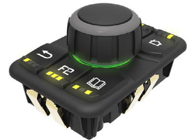
Digital Joystick with 20-Position Continuous Rotation
