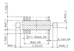
Note 1. Shaded area must be free of any electrically conductive traces to avoid contact with soldered pin header terminations.
