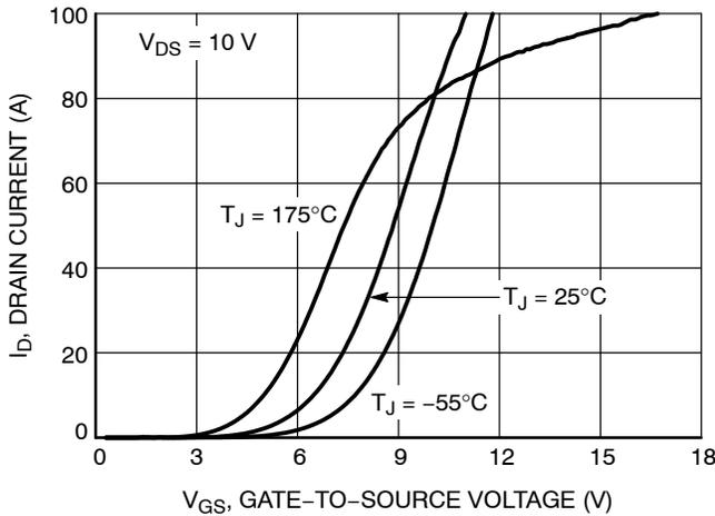
Figure 5. Transfer Characteristics
