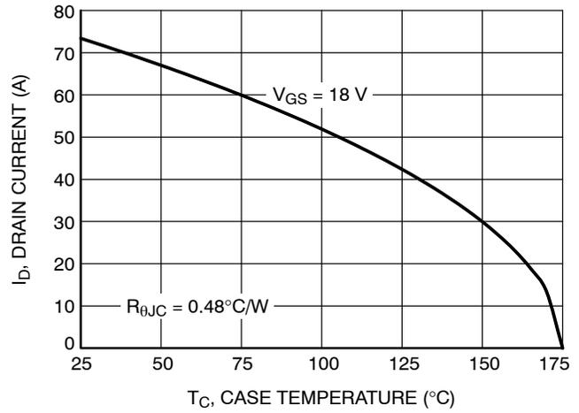
**Figure 14. Maximum Continuous Drain Current vs. Case Temperature**
