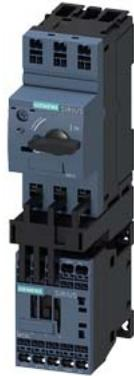
Load feeder fuseless, Direct-on-line starting 400 V AC, Size S00 0.55...0.80 A 230 V AC Spring-type terminal for installation on standard mounting rail (also fulfills type of coordination 1) Type of coordination 2, I<sub>q</sub> = 150 kA 1 NO (contactor)
