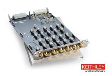
The 3761 provides quality low-current switching at an affordable price. The offset current error generated is specified <1pA, with typical performance at <30fA. When used with a voltage source and an electrometer or picoammeter, this card can easily automate insulation resistance tests, reverse leakage tests on semiconductor junctions, or gate leakage tests on FETs.
