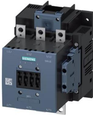
Contactor, AC-1, 275 A/690 V/40 °C, S6, 3-pole, 42-48 V AC/DC, with varistor, 2 NO+2 NC, Connection rail/ screw terminal
