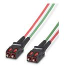
Assembled FO cable, breakout cable, 200/230  $\mu m$  PCF fiber, SC-RJ/IP20 to SC-RJ/IP20, for installation inside control cabinets, length: 5 m
