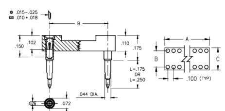
**Description:** DIP Socket Solderless Press-Fit Standard Open Frame Through Hole Accepts .015-.025" Leads **Plating Code:** 13 **Shell Plating:** 10 μ" Gold over 100 μ" Nickel
