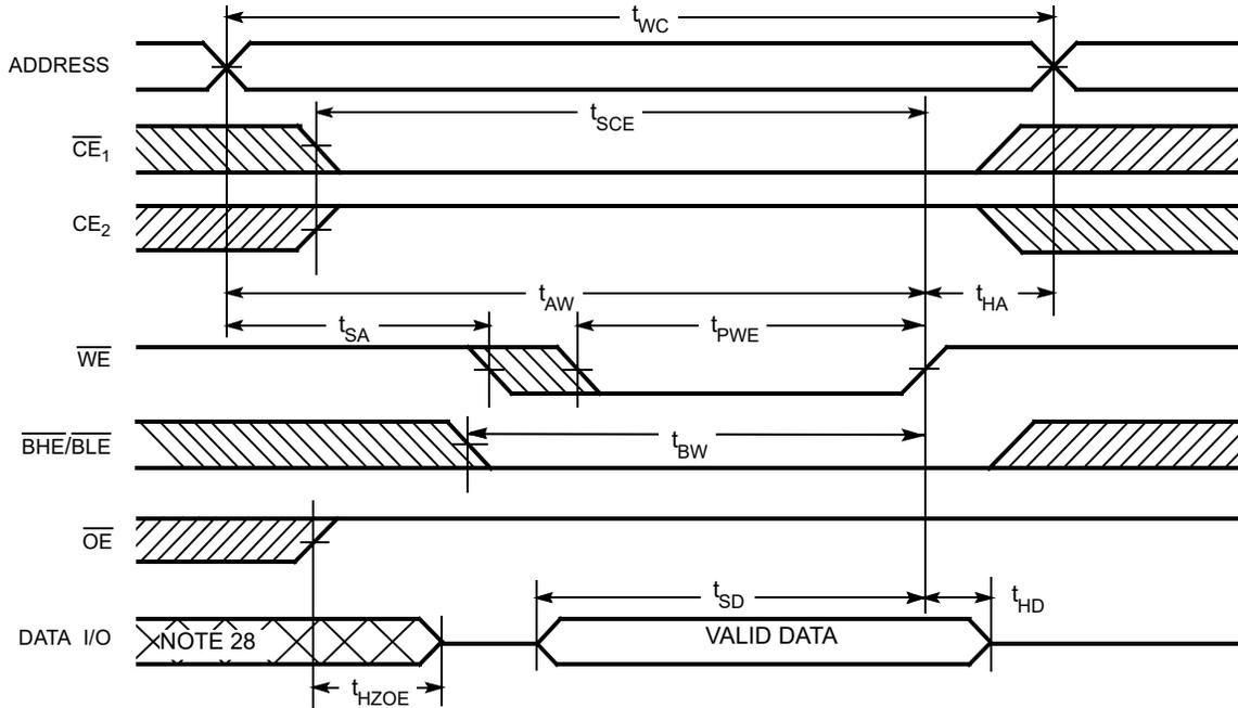
Figure 8. Write Cycle No. 2 ( $\overline{CE}_1$  or  $CE_2$  Controlled) [25, 26, 27, 28]
