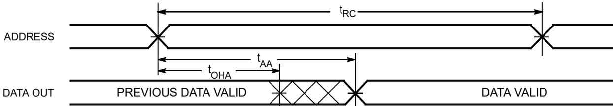
Figure 6. Read Cycle No. 2 ( $\overline{OE}$  Controlled) [23, 24]
