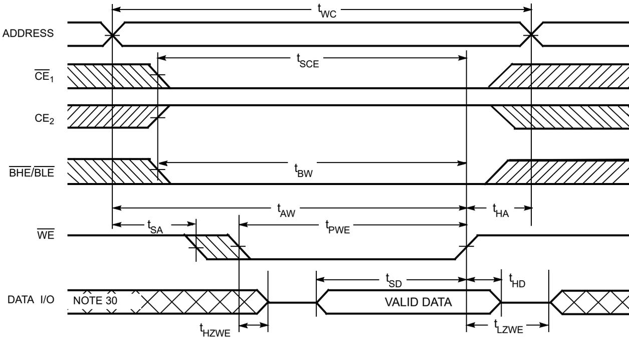
Figure 10. Write Cycle No. 4 ( $\overline{BHE}/\overline{BLE}$  Controlled,  $\overline{OE}$  LOW) [29, 32]
