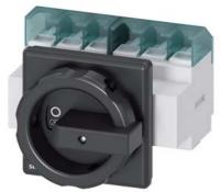
SENTRON, Switch disconnector 3LD, main switch, 6-pole, lu: 63 A, Operating power / at AC-23 A at 400 V: 22 kW, front-mounted, rotary operating mechanism, black, 4-hole mounting of the handle
