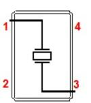
Pad 2 and Pad 4 are common and connected to the metal cover. They are not connected to the crystal.
