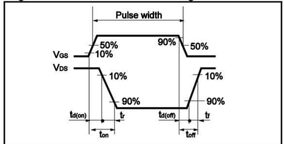
Fig.2-3 Waveforms for Switching Energy Loss
