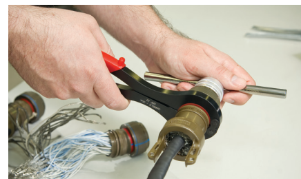
Circular Ring Pliers, strain relief, connector, adaptor, T-handle
