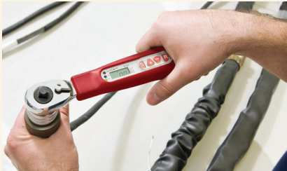
Digital torque wrench, adaptor, connector, strain relief
