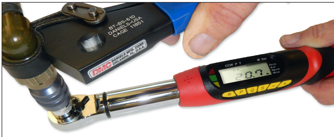
Typical Application - Torque Tightening a Connector Assembly
