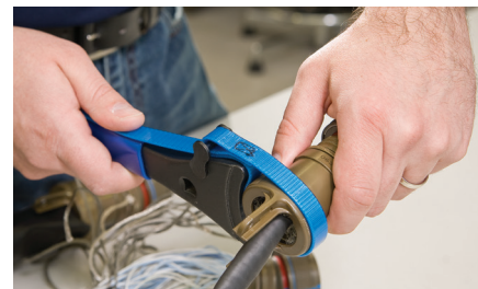
Strap wrench, strain relief, connector
