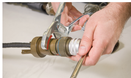
Soft jaw pliers, strain relief, connector, adaptor, T-handle
