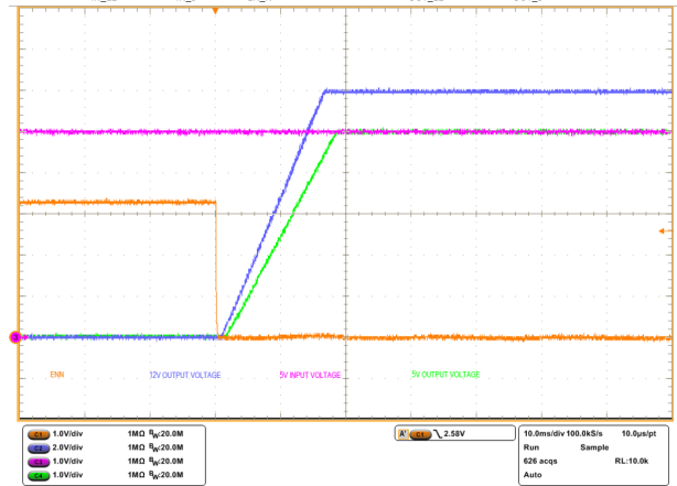
Figure 30. Startup into voltage clamp (5 V eFuse)
