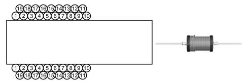
The winding pitch is equal to the wire diameter. The coil is wound with several layers. This leads to parasitic capacitances between the layers in addition to the turn-to-turn capacitances. In comparison to all other types of winding, this type leads to the highest capacitances and thus the lowest resonance frequencies.
