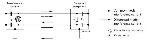
Fig. 8 Common-mode and differential-mode interference
