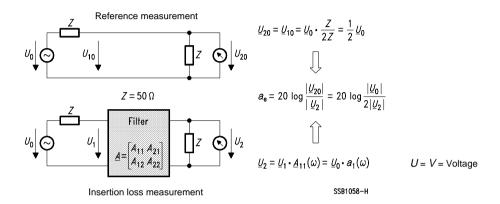
Fig. 12 Definition of insertion loss
