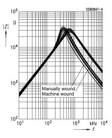
Fig. 14 Impedance |Z| versus frequency *f*Reproducibility and scatter achieved by manual and by machine winding techniques.
