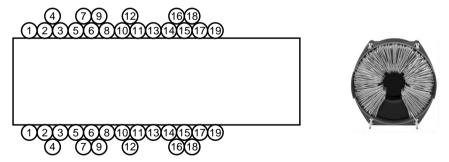
The winding pitch is smaller than the wire diameter. The coil is wound in one direction only. This method of winding a coil does not permit the final position of a turn to be predetermined exactly. The cross section of this type of winding clearly shows a disorderly, "random" arrangement of the turns. This leads to the parasitic capacitances being only minimally greater than those achieved by singlelayer winding, and the resonance frequencies are equal to those achieved by single-layer winding.
