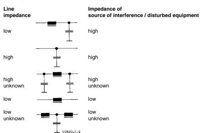
Fig. 9 Filter circuits and impedance relationships
