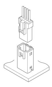
This JWPF connector can be used for the place of which especially waterproof is required.
