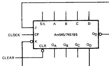
12-BIT SHIFT-LEFT, SHIFT-RIGHT, PARALLEL-LOAD REGISTER
