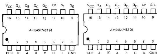
Note: Pin 1 is marked for orientation.
