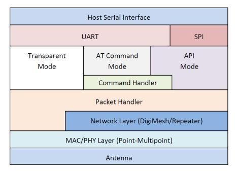
The command handler is the code that processes commands from AT Command Mode or Application Programming Interface (API) Mode (see AT commands). The command handler also processes commands from remote radios (see Remote AT commands).
