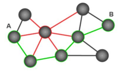
With mesh networking, the distance between two nodes does not matter as long as there are enough nodes in between to pass the message along. When one node wants to communicate with another, the network automatically calculates the best path.
