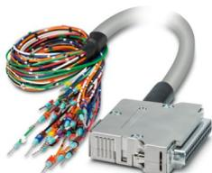
Assembled shielded round cable; connection 1: Single wires (37-position) (The wires are marked and fitted with ferrules); connection 2: D-SUB socket strip (1x 37-position); cable length: 3 m
