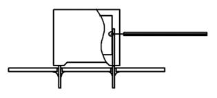
Temperature monitored inside the capacitor.
