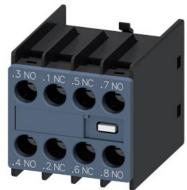
auxiliary switch, on the front, 2 NO + 2 NC, 11 U, .3/4, .1/.2, .5/.6, .7/.8, current path: 1 NO, 1 NC, 1 NC (lagging), 1 NO (leading), screw terminal, for contactors 3RT2 and contactor relays 3RH2
