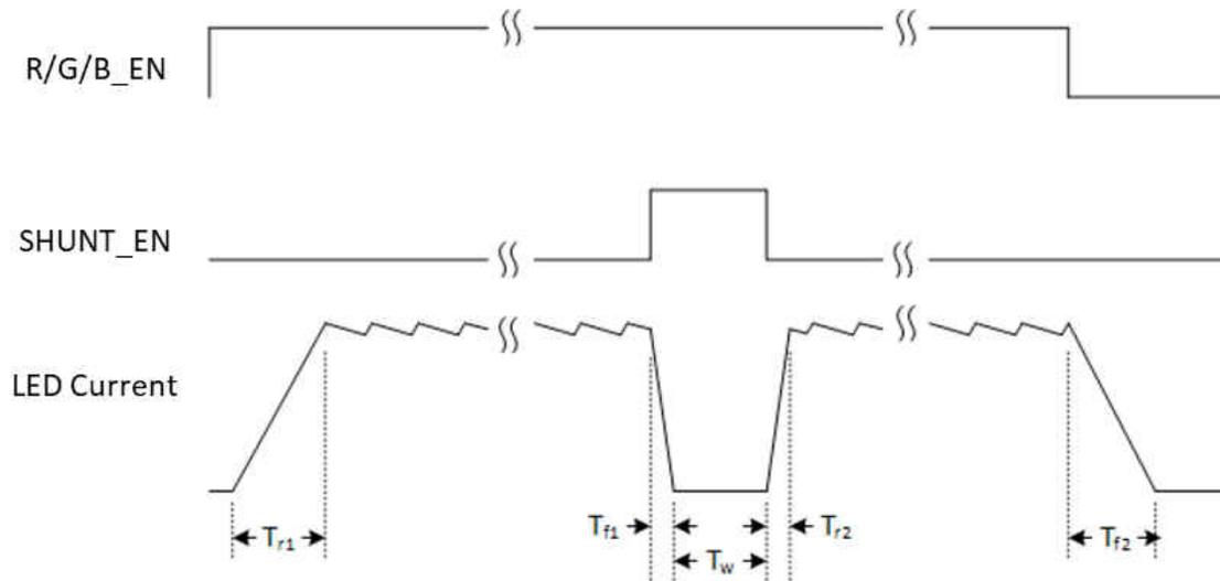
**Figure 2-6. LED Driver Timing Specifications**
