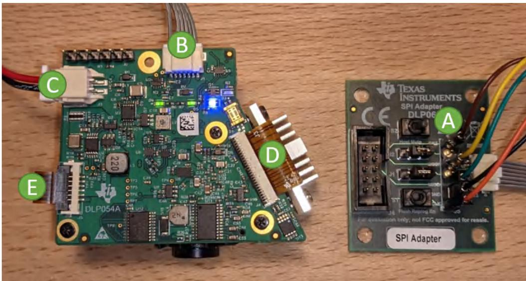
**Figure 3-2. Assembled DLP3021-Q1 Light Engine EVM with FTDI**
