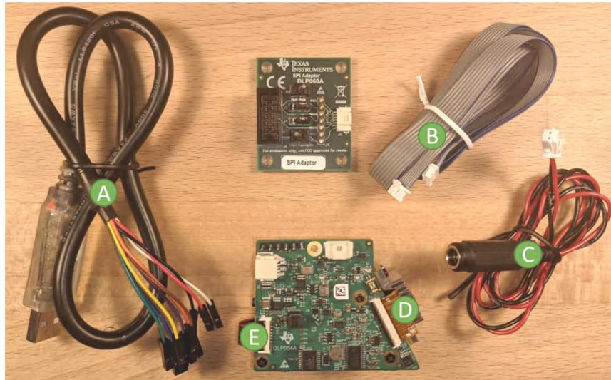
Figure 2-5. Cables Included in DLP3021LEQ1EVM for FTDI
