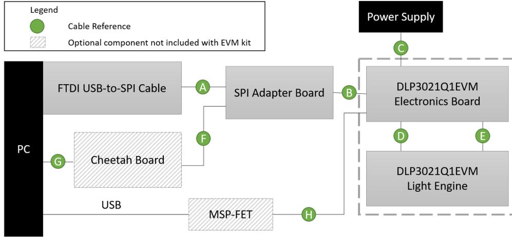
**Figure 3-1. Cable Connections**
