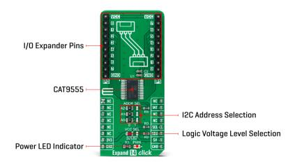
Each I/O port is 5V input tolerant, with a high current I/O drive sink of up to 25mA and an I/O source of up to 10mA, maximum. Additionally, each I/O port is compatible with logic thresholds of 2.5V, 3.3V, and 5V.
