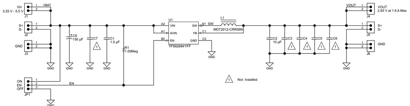
Figure 1. TPS62684EVM-647 Schematic
