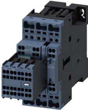
Power contactor, AC-3 32 A, 15 kW / 400 V 2 NO + 2 NC, 110 V DC 3-pole, size S0 Spring-type terminals Removable auxiliary switch
