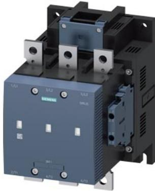
Vacuum contactor, AC-3 300 A, 160 kW / 400 V AC (50-60 Hz) / DC operation 575-600 V UC Auxiliary contacts 2 NO + 2 NC 3-pole, Size S10 Busbar connections Drive: conventional
