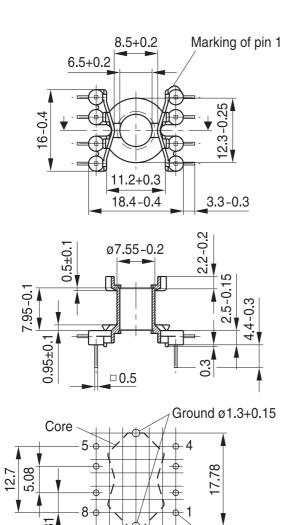
Hole arrangement View in mounting direction
