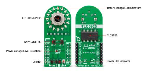
The EC12D1564402 is a 15-pulse incremental rotary encoder with a push button. This encoder has unique mechanical specifications (debouncing time for its internal switches goes down to 2ms), and it can withstand a huge number of switching cycles, up to 30.000. The supporting debouncing circuitry allows contacts to settle before the output is triggered fully.
