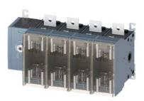
Switch disconnector with fuse 630 A, Size 5, 4-pole for LV HRC fuse Sz. 2 and 3 Front operating mechanism left Basic unit without handle flat terminal
