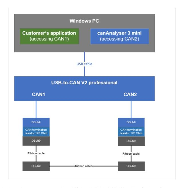
2. Connecting a device or system to the available SUB-D9 of the included cable, with gender changer if required.
