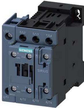
Contactor, AC-1, 35 A/400 V/40 °C, S0, 4-pole, 125 V DC, 1 NO+1 NC, screw terminal
