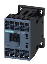
power contactor, AC-3e/AC-3, 9 A, 4 kW / 400 V, 3-pole, 24 V DC, auxiliary contacts: 1 NC, spring-loaded terminal, size: S00, upright mounting position
