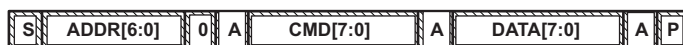
Figure 6. Attempt To Write a Read-Only Address (Nack After Data Sent By Master)
