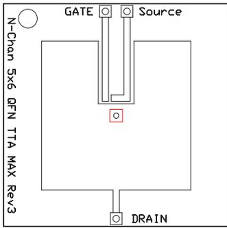
Max  $R_{\theta JA} = 50^{\circ}\text{C/W}$
