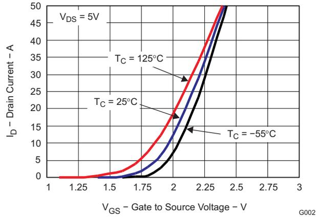
**Figure 3. Transfer Characteristics**
