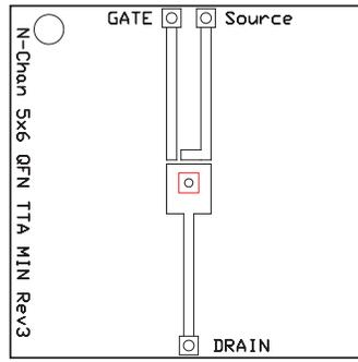
Max  $R_{\theta JA} = 123^{\circ}\text{C/W}$
