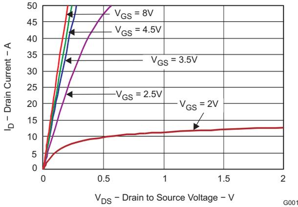
**Figure 2. Saturation Characteristics**
