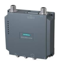
IWLAN access point, SCALANCE W778-1 M12 EEC, 1 radio, 2 N-CON antenna port, iFeatures support via key plug, IEEE 802.11a/b/g/h/n, 2.4/5 GHz, gross data rate 300 Mbit/s, 2x M12 max. 100 Mbit/s, PoE integrated 2-port switch, redundant 24 V DC, M12 A-coded IP65, -30... 70 °C, plug slot WPA2/802.11i/e,conformal coating EN 50155, EN 45545, observe national approvals! CERT ID: MSN65-W1-M12-E2 Scope of delivery: Manuals on CD-ROM, English/German; M12 sealing caps, for operation in the USA
