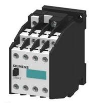
Contactor relay, 62E, DIN EN 50011, 6 NO + 2 NC, screw terminal AC operation 42 V AC 50 Hz/50 V AC 60 Hz
