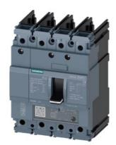
circuit breaker 3VA5 UL frame 125 breaking capacity class S 25kA @ 480V 4-pole, line protection TM230, FTAM, In=125A overload protection Ir=125A fixed short-circuit protection Ii=5...10 x In N conductor protection 100% without connection
