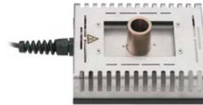
The WSB 80 is a very useful rework preparation tool. The solder bath is temperature controlled continuously from 50°C to 450°C via an existing 80 W power source. The solder bath can be used to tin wire ends and clean leads of all extraneous solder particles in preparation for reworking. (Usable for lead free solder.)
