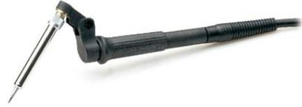
An 80 W Antistatic Peritronic soldering pencil that gives all-round vision when making intricate connections. Antistatic cord and handle. Electronically temperature controlled. Consists of MPR 80 Antistatic and KH 25P Support.
