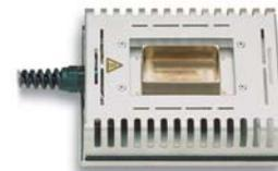
The WSB 150 solder bath is optimally suited to tin coating and preparation of soldering components. It has a temperature range of 50°C–550°C with heat output of 150 W, making the WSB solder bath an ideal accessory to the Weller WSD 150 soldering station. To guard against dripping solder residue, the solder bath is placed in a V2A tray, supplied as an optional extra. (Usable for lead free solder.)
