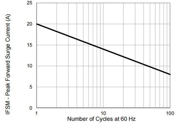
Fig.6 - Maximum Non-Repetitive Peak Forward Surge Current Uni-Directional Only
